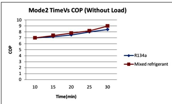
Fig. 4. Mode 2 Time Vs COP (Without Load)
