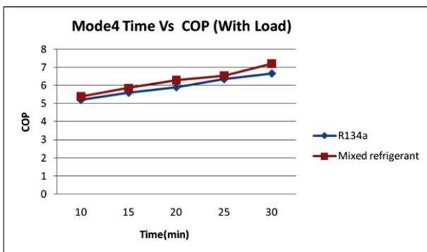
Fig. 10. Mode 4 Time Vs COP (With Load)
