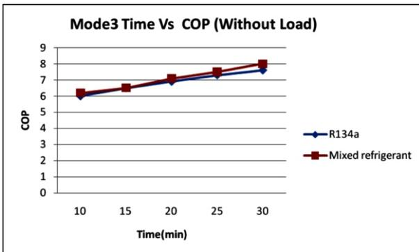
Fig. 5. Mode 3 Time Vs COP (Without Load)
