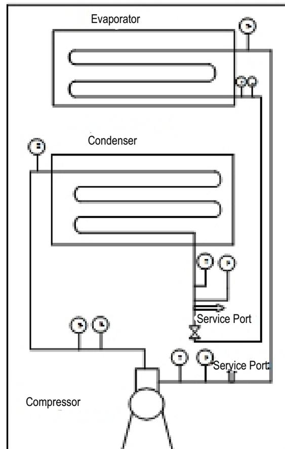
Fig. 2. Schematic diagram of the investigation unit and apparatus
