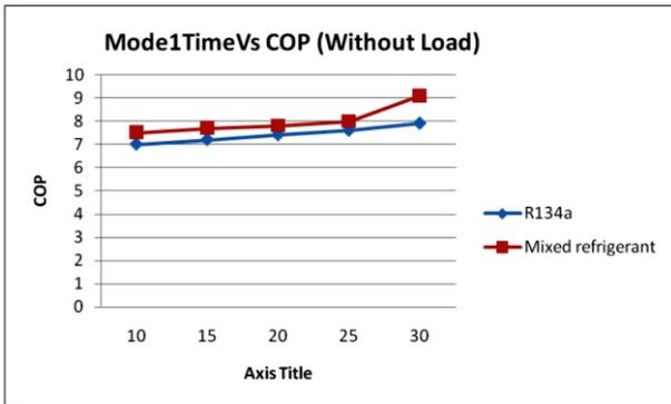
Fig. 3. Mode 1 Time Vs COP (Without Load)
